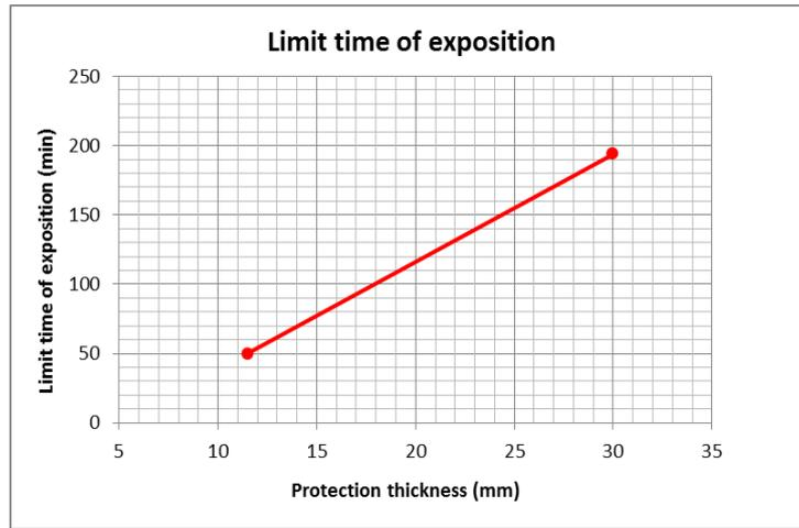
**Insulation.** The thermal insulation of the mixed slab + the protection according to EN 1363-1 is:
