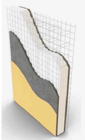
Figure 1. Panel – Factory made 3-dimensional grid of steel wires and a core of thermal insulation material of expanded polystyrene, EPS, plus concrete applied by shotcrete technique. (Example)
