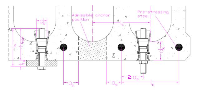
h<sub>nom</sub>: Overall anchor embedment depth in the base material
